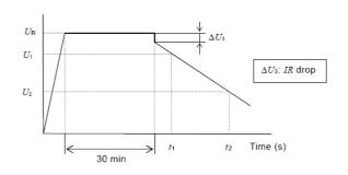
$$C = \frac{I \times (t_2 - t_1)}{U_1 - U_2}$$
